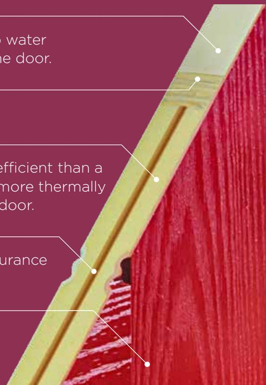
Our composite doors combine glass-reinforced plastic skins with a polymer frame to create a rigid door structure. In addition, an engineered timber frame adds further strength and rigidity to the door along with a reinforced central core for security.
